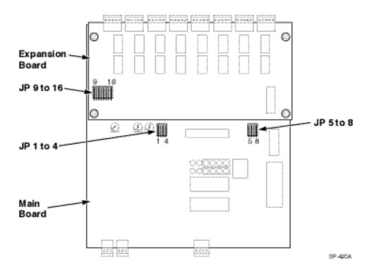
Figure 4. Communications Controller Jumpers
